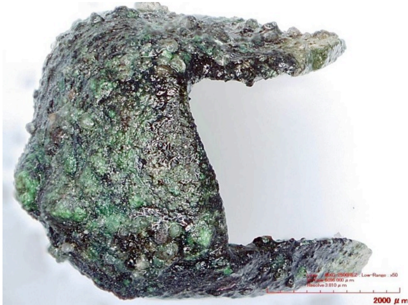
Photo 3. Photo taken with a HIROX microscope. Gloss and grains of cyanoacrylate.
