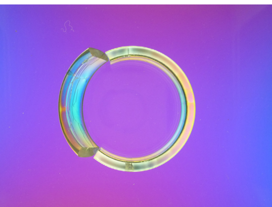
Figure 6 Bracelet viewed under Sharples strain viewer
