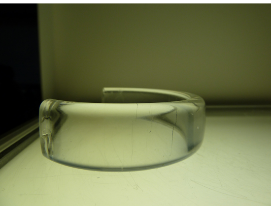
Figure 7 Stress cracked bracelet from RCE reference collection
